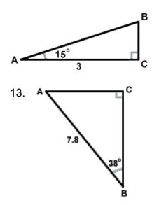
If we know the sides, we can determine the angles. In the triangle above, if we know AC and AB, we know the sine of angle ABC is AC/AB (opposite over hypotenuse). So the angle ABC is sin<sup>-1</sup> (AC/AB).
